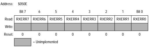
Figure 24. Receiver Error Counter (CRXERR)
