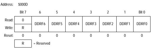
Figure 18. Data Direction Register F (DDRF)
