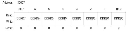
Figure 12. Data Direction Register D (DDRD)
